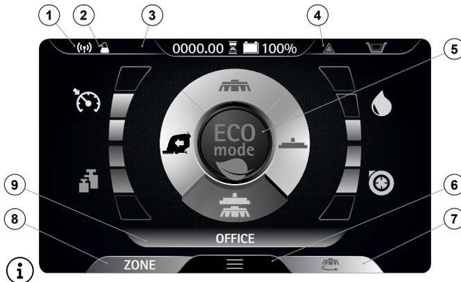
By selecting the "SCRUBBING WITH DRYING" program, the command display screen will appear as in the adjacent figure.
