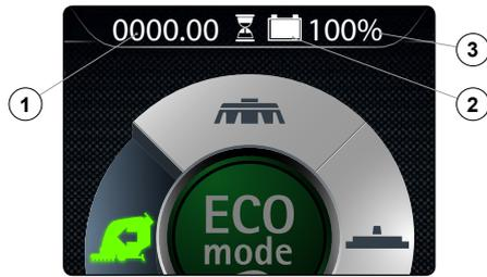
The control display is in the control panel, at the top in the middle it is possible to observe the total time the machine has been used.
