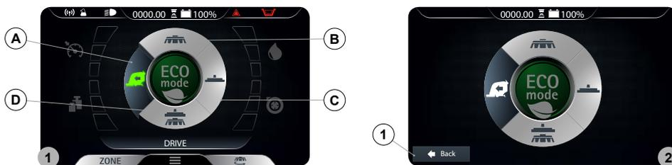
**! ATTENTION:** if you want to pass from a work program with the washing mode (only washing or washing with drying) to the transfer program always remember to select the vacuum program for the time needed to collect the detergent solution on the ground.
