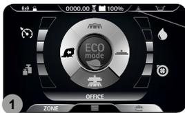
When an error occurs the symbol (1) is displayed in the information field (**Fig. 1**), it remains visible until the error is resolved.
