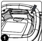
1. Press the "REVERSE ACTIVATION - DEACTIVATION" button (1) on the control handlebars (**Fig.1**).
