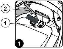
The machine has an automatic service for activating an urgent technical assistance request. To activate this function, the operator has to press the button (2) under the hatch (1) bearing the symbol "SOS" (Fig. 1).
