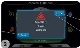
**i** **N.B.:** to close the error screen press the button (3) (**Fig.2**).
