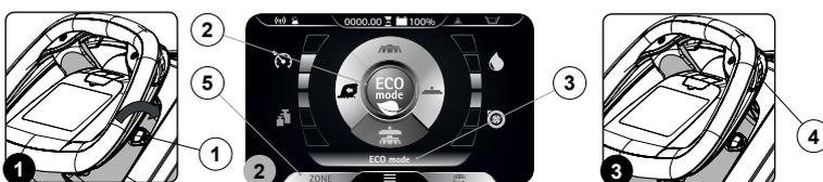
**i** **N.B.:** if the button (2) is pressed when working in ECO-MODE, the machine will shift to MANUAL MODE, leaving the program in use at the time active (**Fig.4**).
