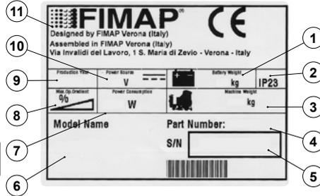
1. The maximum weight of the batteries that power the machine (expressed in kg).
