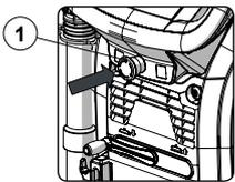
If any serious problems are encountered during the work operations, press the battery disconnect button (1) on the electrical system carter.
