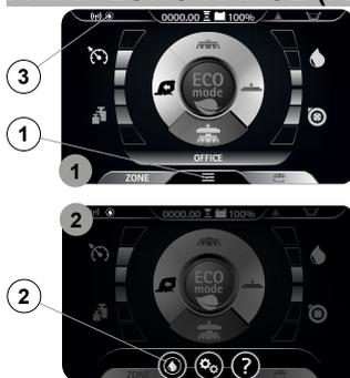
1. With the machine on, press the menu button (1) on the working screen (Fig.1).
