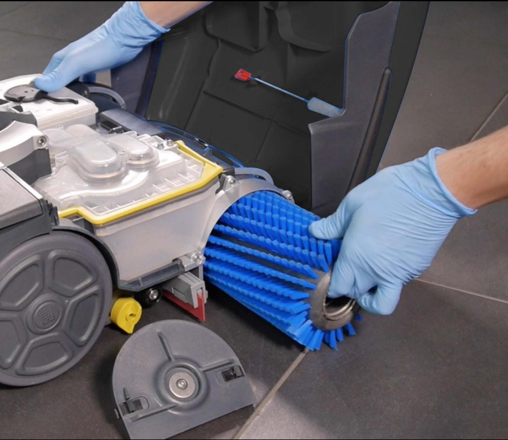
The brush is easy to remove without any tools for maintenance operations
