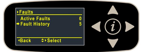
Each fault is displayed along with; (Nx) where "N" is the number of times the fault has occurred, the timestamp shows the most recent occurrence and description. Use the up and down arrows to scroll through the list of faults.
